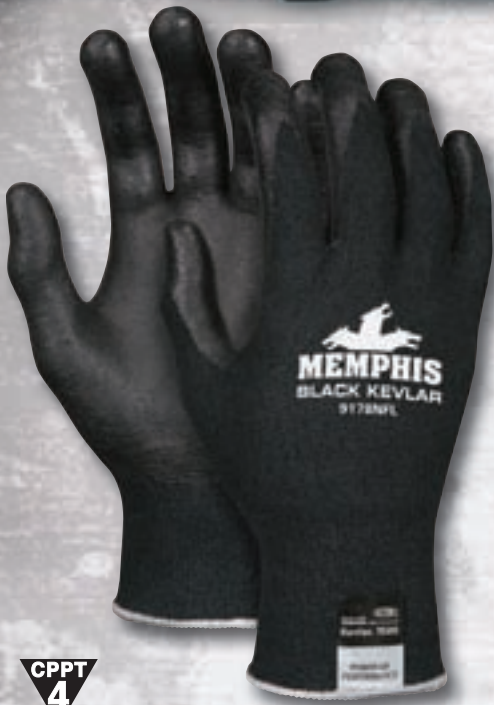
9178NF Black KEVLAR® Sizes: S-XL 13-Gauge Black KEVLAR®/Synthetic Shell with Black Nitrile Foam Coating on Palm and Fingertips. CE 4542, CPPT level 4.
