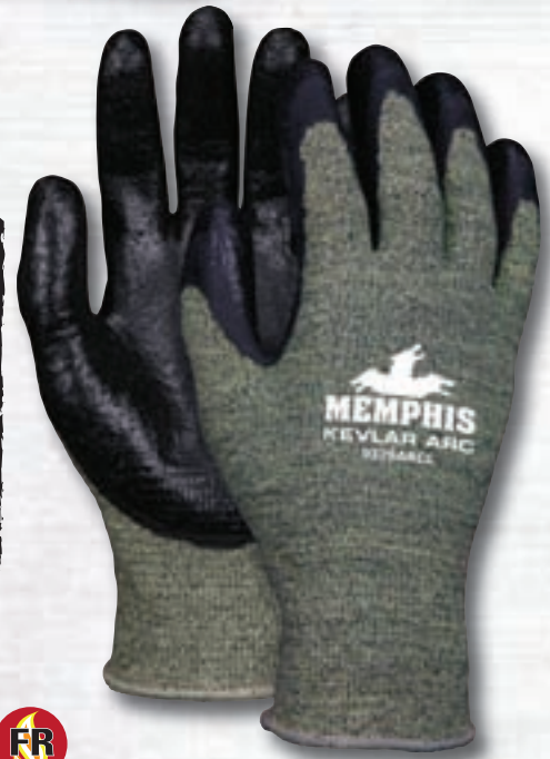
9379ARC KEVLAR® ARC Sizes: S-XXL 13-Gauge Speckled Green/Black KEVLAR®/Synthetic Shell with Black APG (Abrasion, Performance, Grip) Coating on Palm and Fingertips. CE 3543, CPPT level 4.
