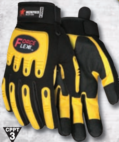
KV200 ForceFlex™ Sizes: M-XXL KEVLAR® Full Sock Lining, Yellow Clarino® Leather Palm Reinforced with Black Textured Palm and Fingertips for Maximum Grip in Oily or Wet Conditions, TPR Exoskeleton Back of Hand Protection, Adjustable Wrist Closure, Black Pull Tab. Great for Cutting Fluids. CPPT level 3.
