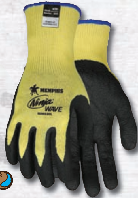
N96930 Ninja® Wave Sizes: S-XXL 10-Gauge KEVLAR® Shell with Black Nitrile Wave Coating on Palm and Fingertips. CE 4343, CPPT 2.
